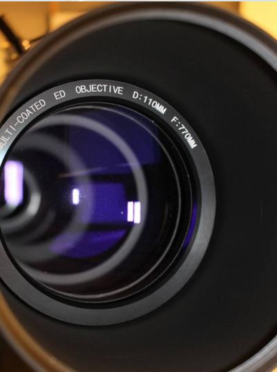
11 cm refractor with low-dispersion glassF: 770mmEquipped with a field correctorStellarVue, USA.
