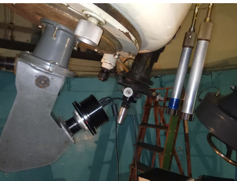
Telescope AZT-14A with the spectrograph ASP-9
